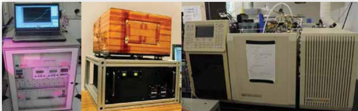
Instruments in the trace gas isotope lab at Biosphere 2 (from left): proton transfer reaction mass spectrometer (PTR-MS), quantum cascade laser absorption spectrometer (QCLAS), and gas chromatograph-ion trap mass spectrometer (GC-ITMS).
